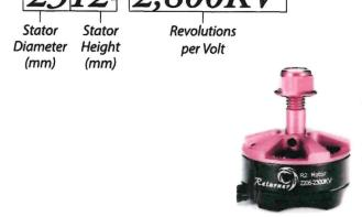
The combination of the motor's stator diameter and height determine its maximum torque value. The motor should be labeled with this information as in the image to the left.
